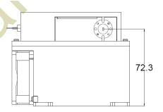
Outline wit heatsink and Fan in default Customer can remove the heatsink and Fan if using their own heatsink system.
